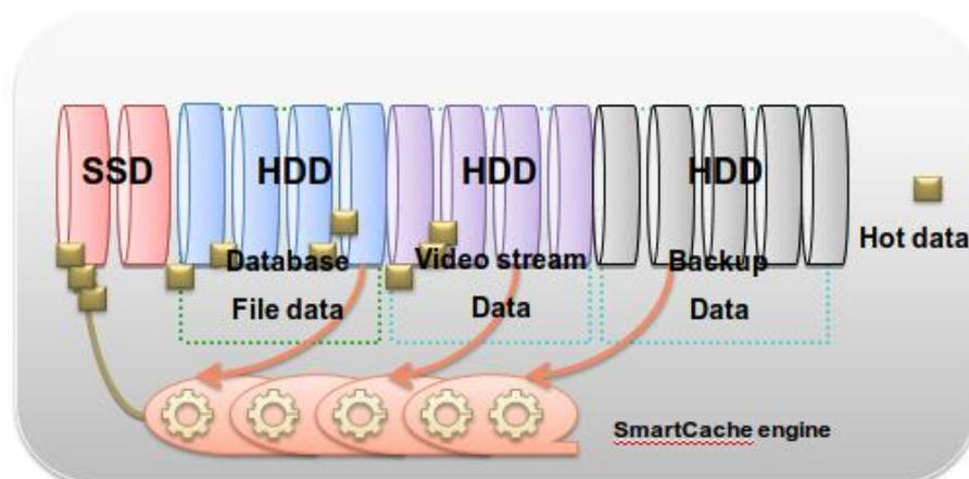
Figure 3-3 SmartCache working mechanism
